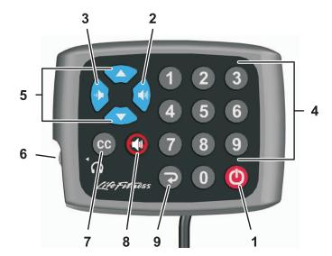
Turn the power on by pressing the ON/OFF key (1) on the remote control. A blue LED appears on the lower right corner of the TV when the power is on. The LED blinks during SLEEP mode (the back light will be off).
